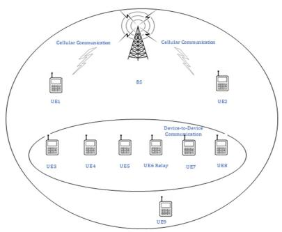
Cellular communication and D2D communication. Both single-hop and multi-hop (including D2D relay) networks formed by D2D links are shown above.
