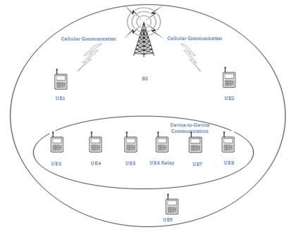
Cellular communication and D2D communication. Both single-hop and multi-hop (including D2D relay) networks formed by D2D links are shown above.
