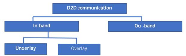
Bias communicates directly with or without the involvement of a BS, eNB, or eNodeB using the D2D conception. D2D links give ultra-low quiescence and high data rate connections between bias in close propinquity. D2D links operate on either certified or unlicensed diapason, as described in the sections Inband and Outband.
