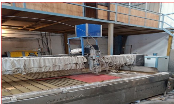
Fig.2 Abrasive water jet machine experimental setup
