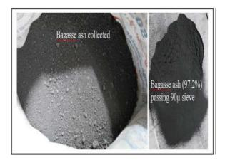
The sugarcane bagasse consists of approximately 50% of cellulose, 25% of hemicellulose and 25% of lignin. Each ton of sugarcane generates approximately 26% of bagasse (at a moisture content of 50%) and 0.62% of residual ash. The residue after combustion presents a chemical composition dominates by silicon dioxide (SiO2)[6]. In spite of being a material of hard degradation and that presents few nutrients, the ash is used on the farms as a fertilizer in the sugarcane harvests.
