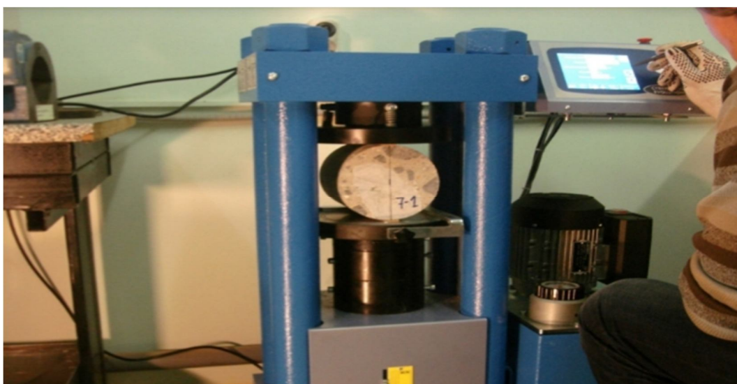
Figure 6. split tensile strength test of cylenders
