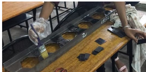
Fig. 9 Applying adhesive on castellated beam
