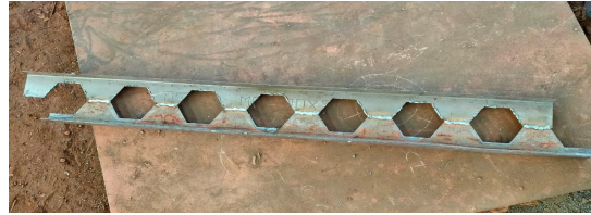
Fig. 7 Final Specimen of castellated beam
