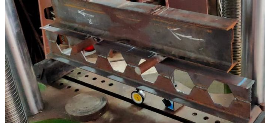
Fig. 12 Test set up of control castellated beam
