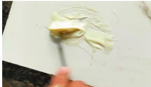
Fig. 8 Mixing of resin with hardener
