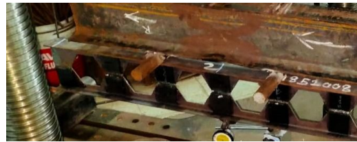
Fig. 13 Test set up of hexagonal castellated beam with transverse CFRP stiffeners
