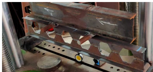
Fig. 12 Test set up of control castellated beam
