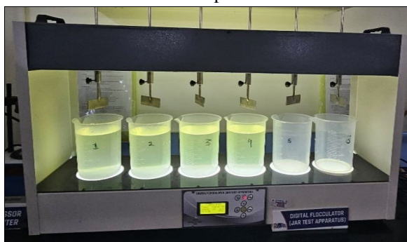
Fig.10. a. Urban Lake Water Sample Before PAC Treatment
