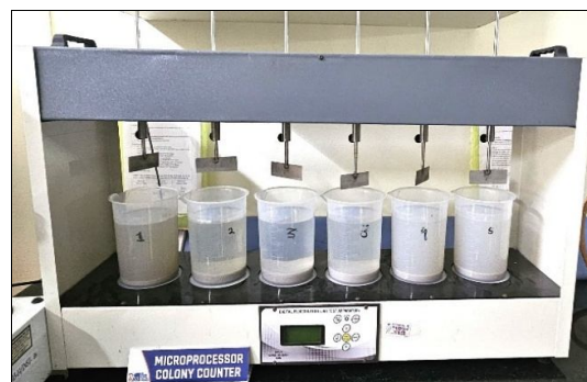
Fig.8.b. Clear Supernatant After PAC Treatment of Domestic Wastewater
