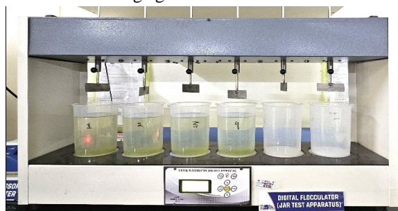
Fig.10.b Clear Supernatant After PAC Treatment of UL water
