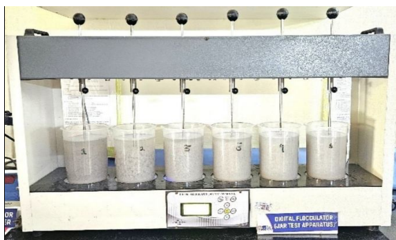
Fig.8.a. Jar Test Showing Floc Formation in Domestic Wastewater Treated with PAC
