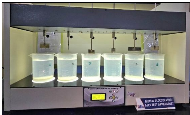
Fig.7. Floc formation and sedimentation observed after treatment of bentonite clay-induced turbid water with Poly Aluminium Chloride (PAC)
