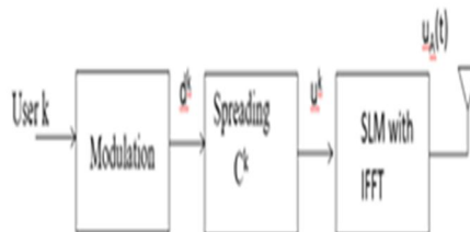
Figure 1: MC-CDMA using SLM
