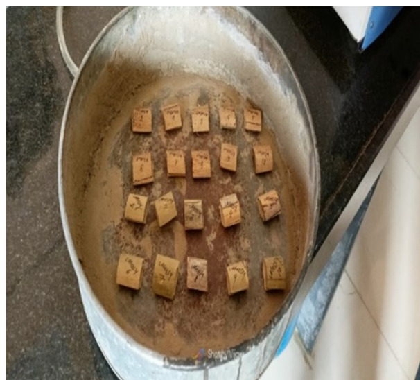
Fig. specimen for Moisture Content
