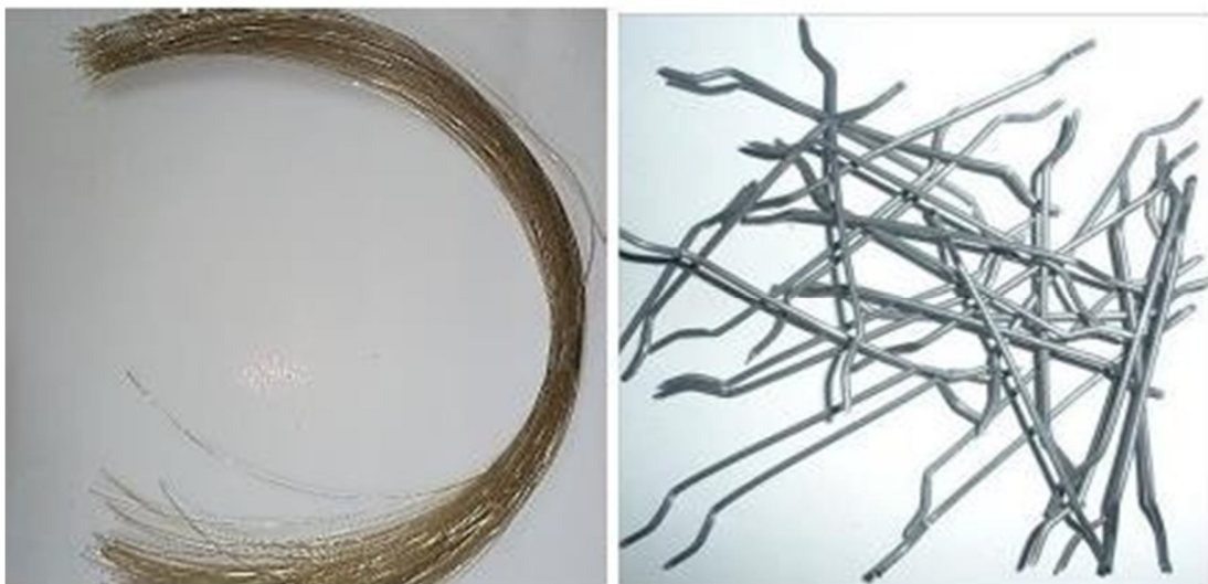
Fig. 5. Synthetic macro nylon fibres (SNF, left) and hooked-end steel fibres (right) used in the study. Nylon fibres: \text{\O} 0.5 \text{ mm} , tensile strength 300 MPa, elongation 14% [3].
