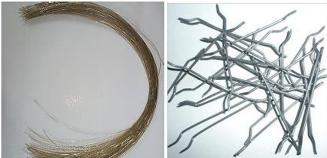
Fig. 5. Synthetic macro nylon fibres (SNF, left) and hooked-end steel fibres (right) used in the study. Nylon fibres: \text{\O} 0.5 mm, tensile strength 300 MPa, elongation 14% [3].
