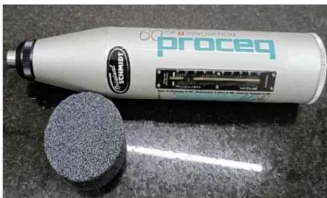
Fig.1: Schmidt Rebound Hammer. [7]
