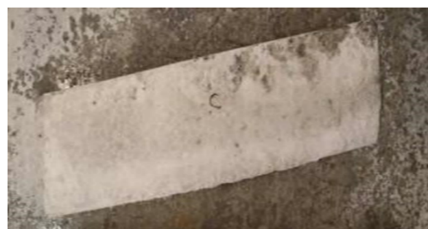
Two point load Reference Beam Specimen
