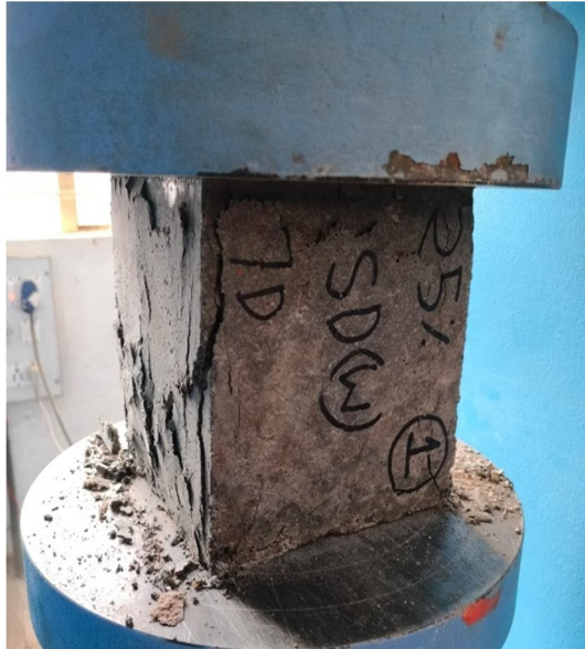
Fig.4.1: Concrete Cube After Test
