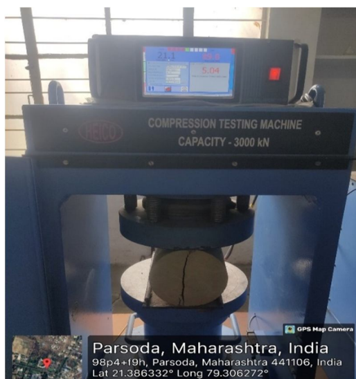
Fig.5.4: Split Tensile Strength Test
