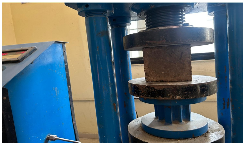
Fig. 5. Compression Testing Machine (CTM) Used for Compressive Strength Testing
