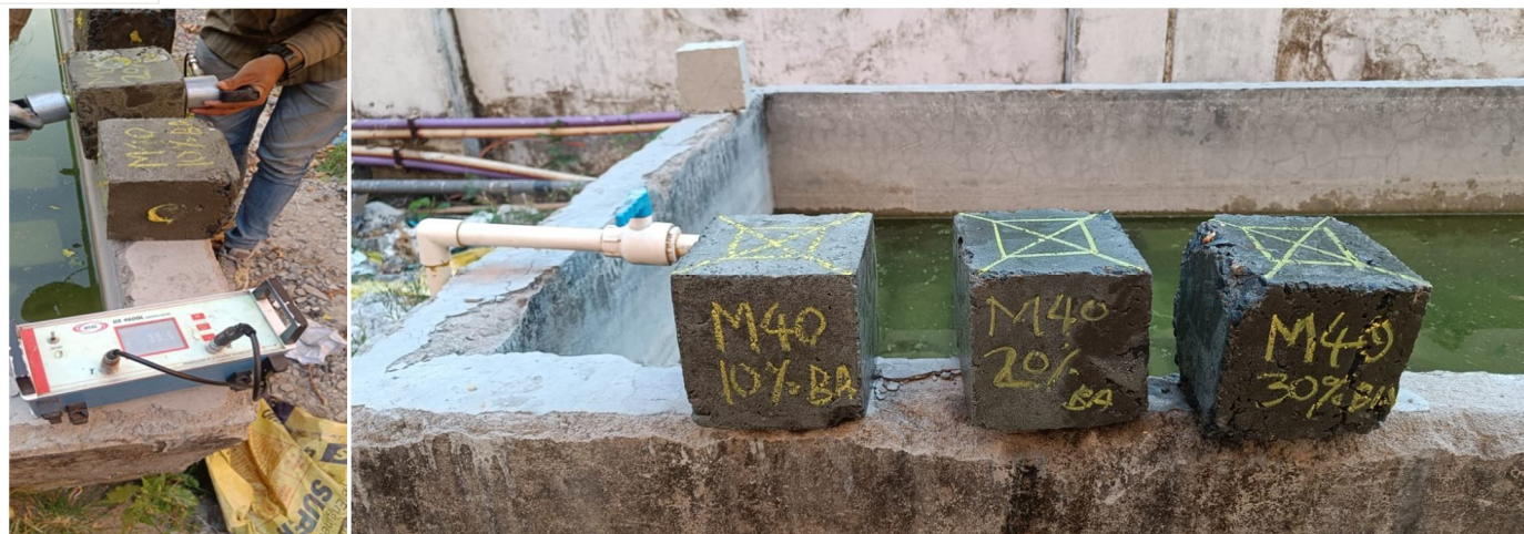
Fig. 6 Ultrasonic Pulse Velocity Measurement on Concrete Cube
