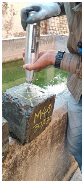
Fig. 7 Rebound Hammer Test Setup for Concrete Specimen
