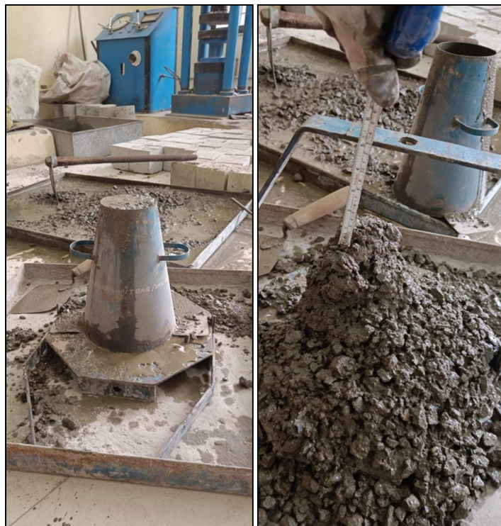
Fig. 2: Slump Cone Apparatus Used for Workability Test
