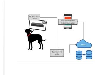
The figure shows the architecture of our project. The device is attached to the collar of the dog and the data from the device is given to the cloud. Then the information is transmitted from the cloud to our app.
