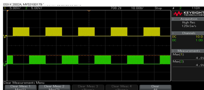
Fig 7: PWM pulse to the SEPIC converter
