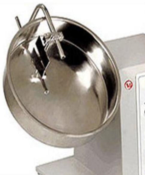
Figure 6. Rotary disk pelletizing equipment
