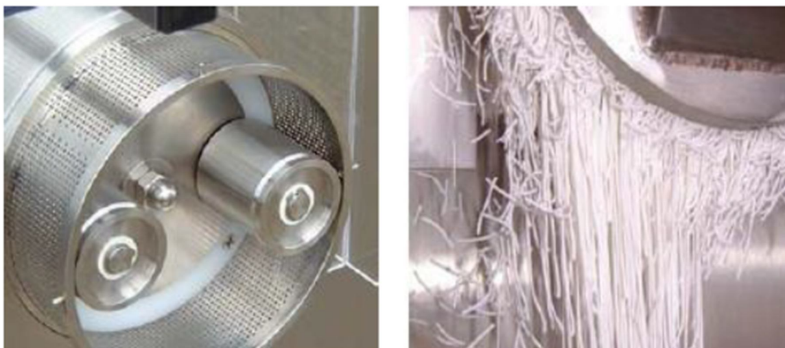
Figure 7. Extruder during operation [77]
