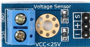
Fig. 5: 25V voltage sensor
