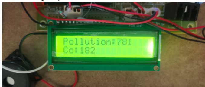
Figure 12. Display showing the safe condition.
