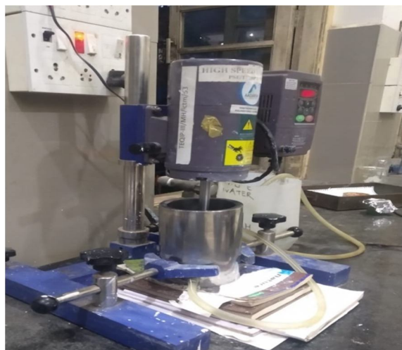
Fig. 2.1 High speed disperser for paint formation
