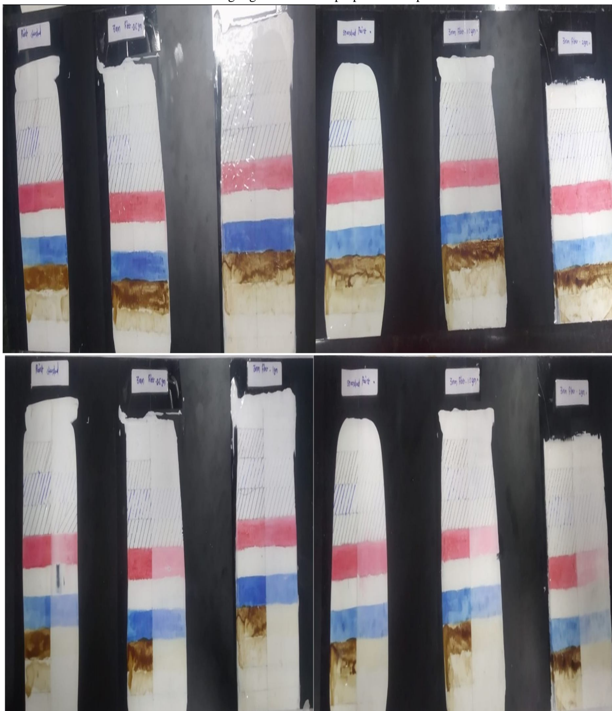
Fig. 5.3 : stain resistance test before and after
