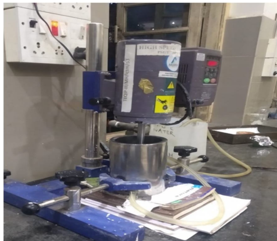
Fig. 2.1 High speed disperser for paint formation
