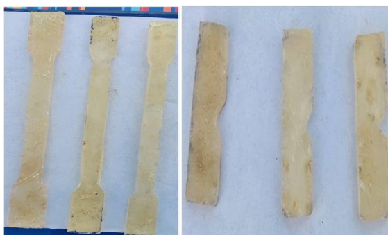
Fig 3: Resin Specimen for Tensile and Impact tests specimen
