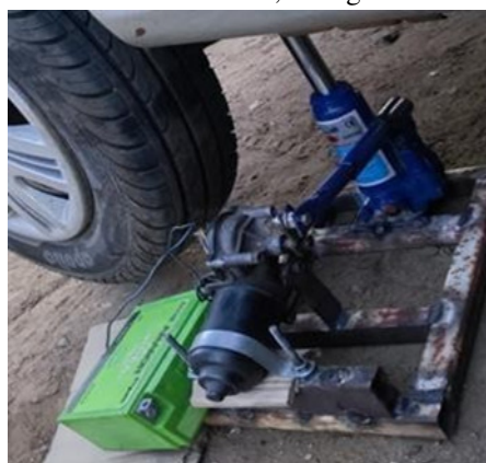
Fig 8. Motorized Hydraulic jack
