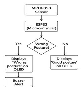
Fig3: Block diagram
