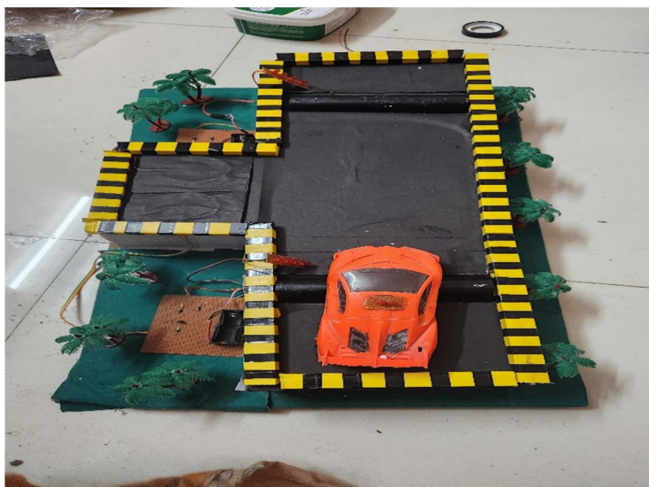
Figure 7 – Car on speed breaker for energy generation
