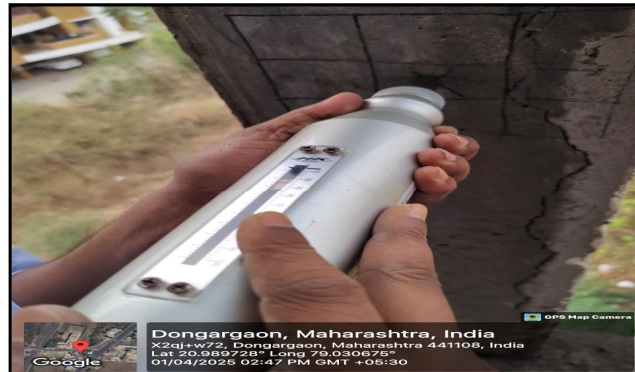
Photo 3 & 4) Rebound hammer testing on column surfaces
