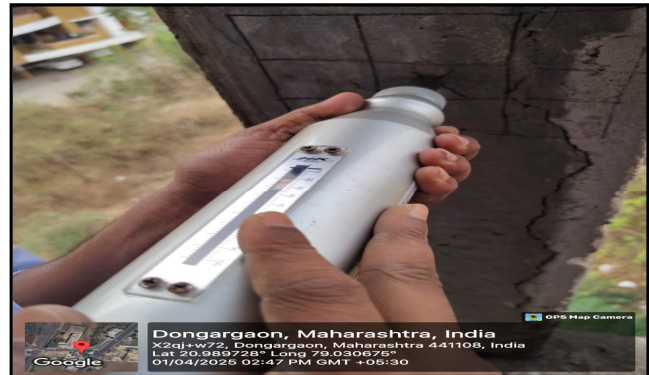
Photo 3 & 4) Rebound hammer testing on column surfaces
