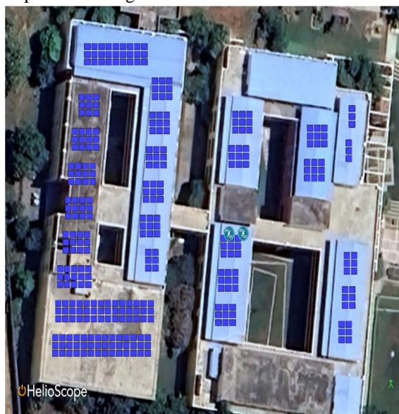
Fig 9 Complete Simulation diagram of the Rooftop Solar PV System using HelioScope .
