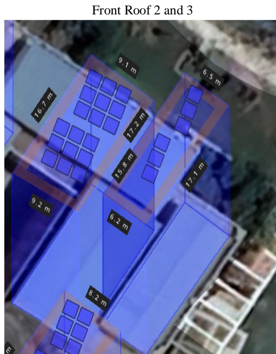
Fig 4 Front Roofs 2 and 3: 6 and 18 modules respectively, Generation of 2 KW and 6KW respectively (The near to front is 2 and back is 3)
