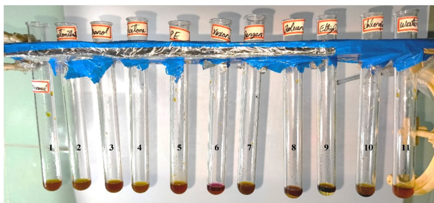
Fig 1. Alkaloids (Wager's Test): 1-Methanol, 2-Acetonitrile, 3-Ethanol, 4-Acetone, 5-Petroleum Ether, 6-Hexane, 7-Benzene, 8-Toluene, 9-Ethyle Acetate, 10- Chloroform, 11- Water
