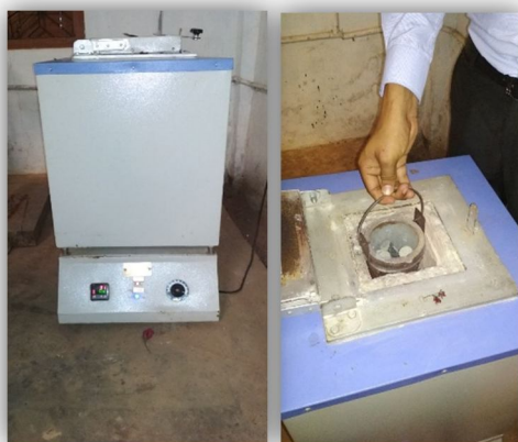
Fig. 7: Muffle furnace used for sintering the compacts
