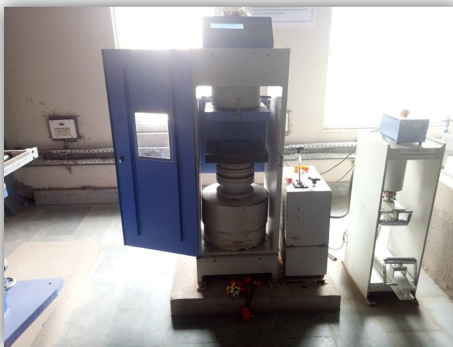
fig. 5: Digital power compaction machine (3000 kN capacity)
