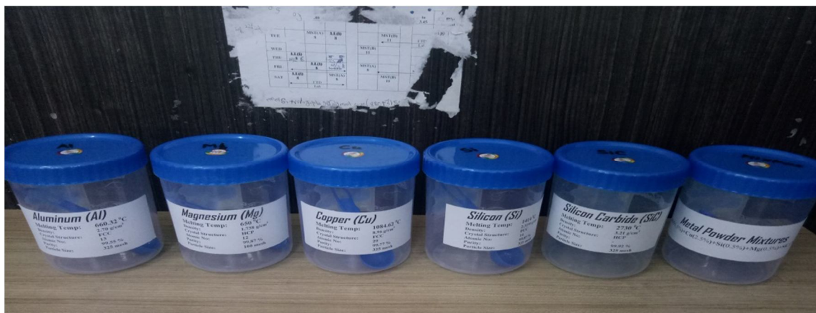
Fig. 1: As–received metal and ceramic powders used in the study
