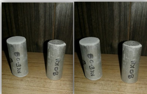
Fig. 6: Green compacts obtained after cold compaction
