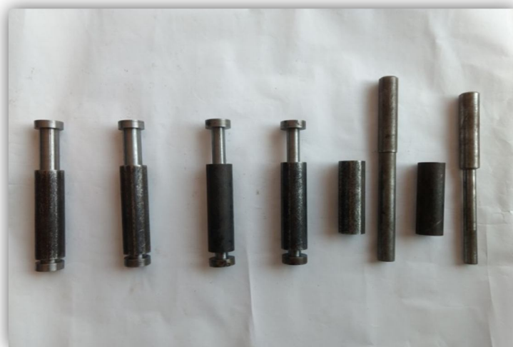
Fig. 3: Finished dies after machining and polishing
