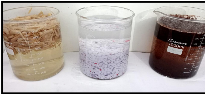
Figure 3.2-Soaked samples (sugarcane bagasse, waste paper and coconut fibre)
