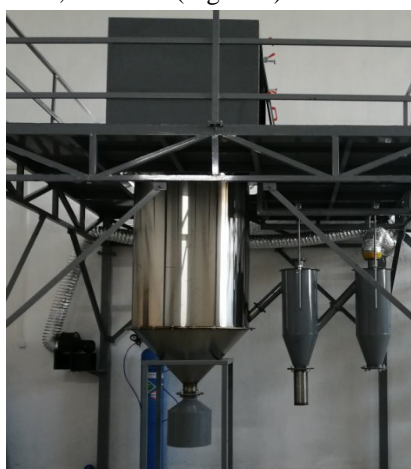
Fig 1. Vertical gas atomization unit designed and manufactured
