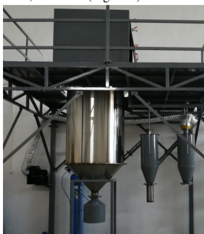
Fig 1. Vertical gas atomization unit designed and manufactured
