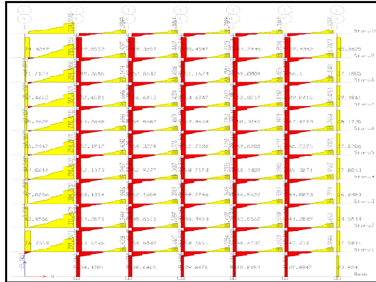
Fig. 5.4: SFD after removal of column C1
