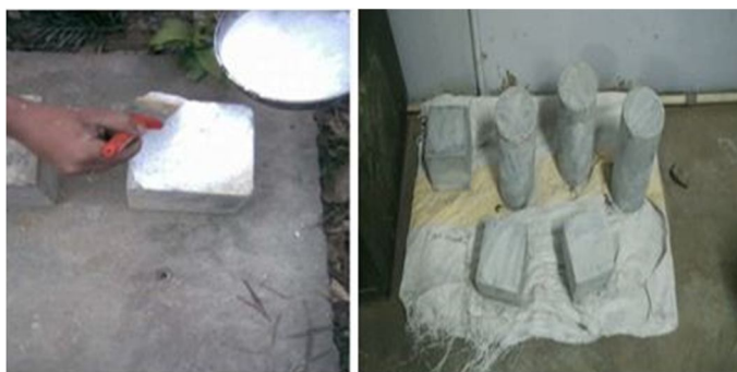
Fig 7. Curing of concrete
