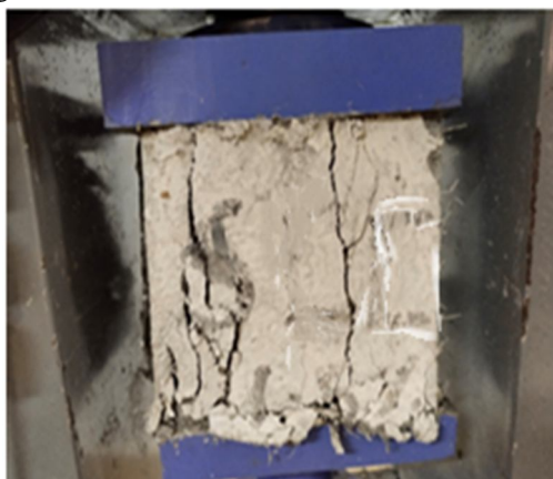
Fig 10. Specimen under compressive test
