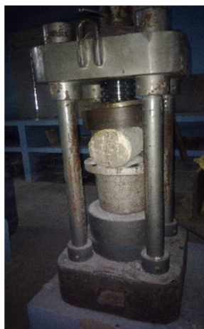
Fig 12. Specimen under Split Tensile Test
