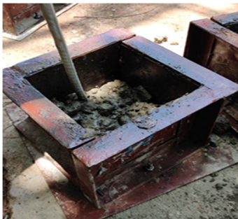
Fig 5. Casting of specimens
