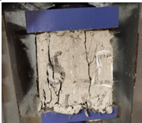
Fig 10. Specimen under compressive test
