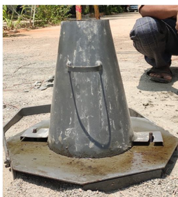
Fig 8. Slump cone test
