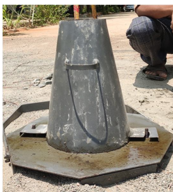
Fig 8. Slump cone test
