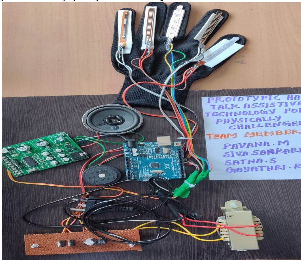
Fig.7. Harware Implementation of prototypic Hand Talk Assistive Technology For Physically Challenged.
