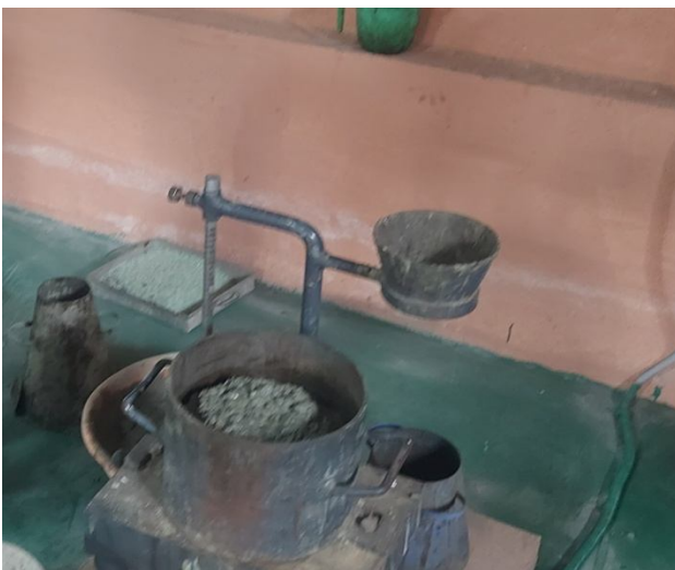
Fig -1: Vee bee consistometer test
