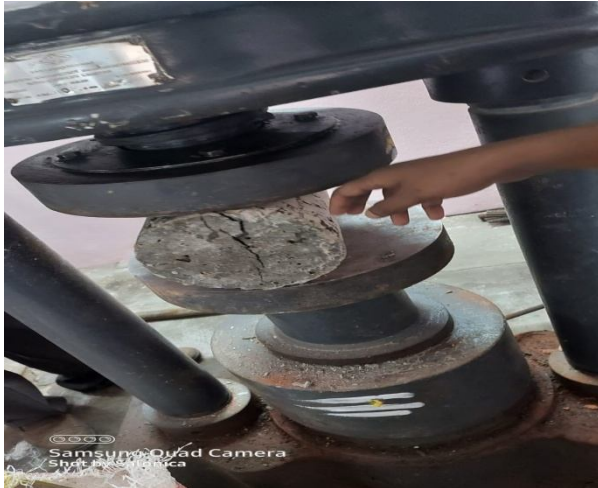
Fig -3: Split tensile test
