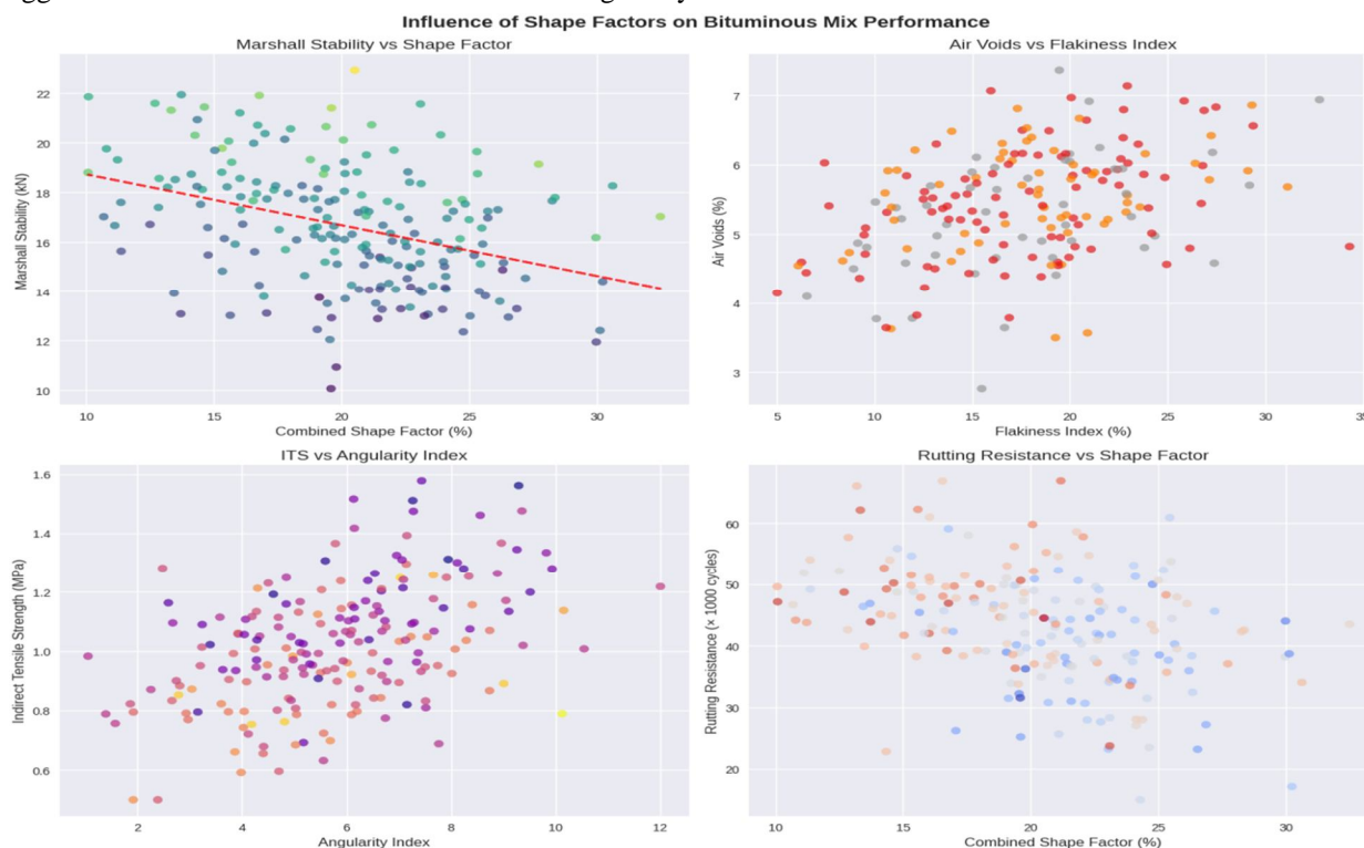
Figure 3. Influence of Shape Factors on Bituminous Mix Performance
