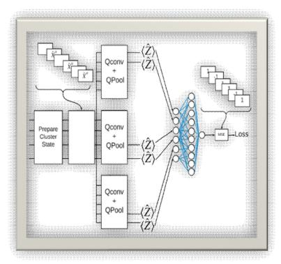
b) Model Architecture with Parameterized Quantum Circuit and Dense Layers:
