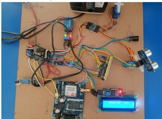
Fig 3: Ultrasonic Sensor detecting the person
