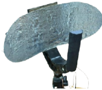
Fig.2. Custom parabolic directional antenna
