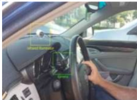
Fig 1: Camera and IR illuminator position.
