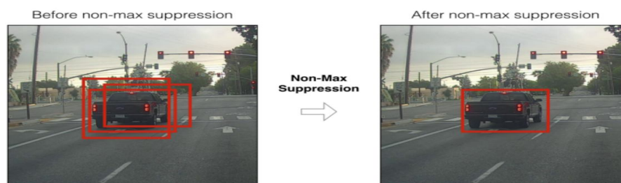
Fig. 2 Before and after Non-Maximum Suppression
