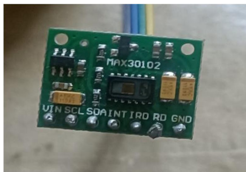
Fig. 4 Pulse Oximeter Sensor
