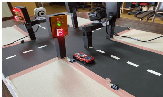
Fig. 5. Traffic lane demonstrating a single sensor trigger
