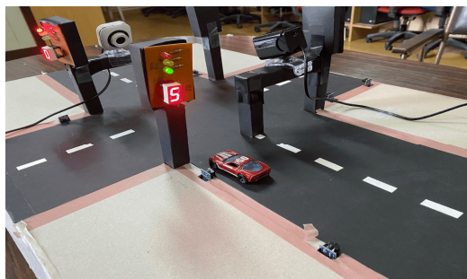
Fig. 5. Traffic lane demonstrating a single sensor trigger
