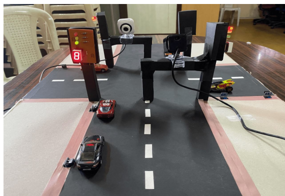
Fig. 6. Traffic lane demonstrating a two sensor trigger
