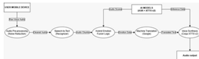
Fig. 2. Detailed processing pipeline highlighting the Hybrid Emotion Fusion logic and component integration.
