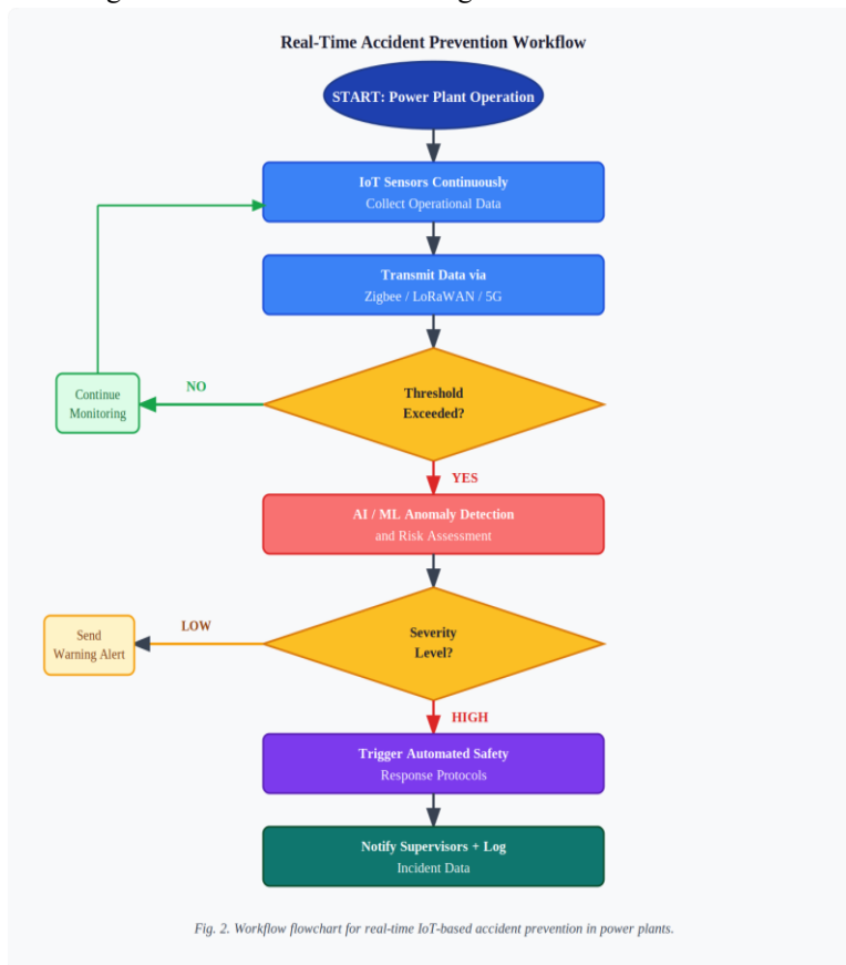
Fig. 2. Workflow flowchart for real-time IoT-based accident prevention in power plants
