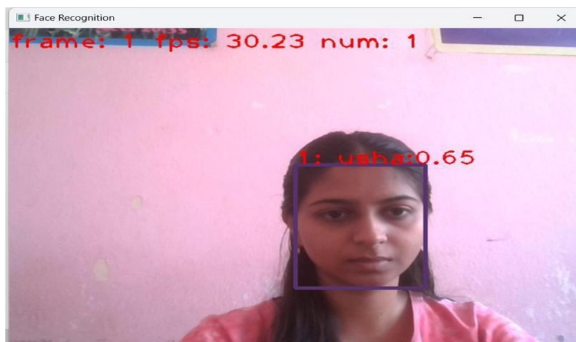
Figure 5: The features are extracted using ArcFace and compared to a known database with the help of the Cosine Similarity algorithm for recognition. The recognized persons will later have confidence scores assigned by the system.
