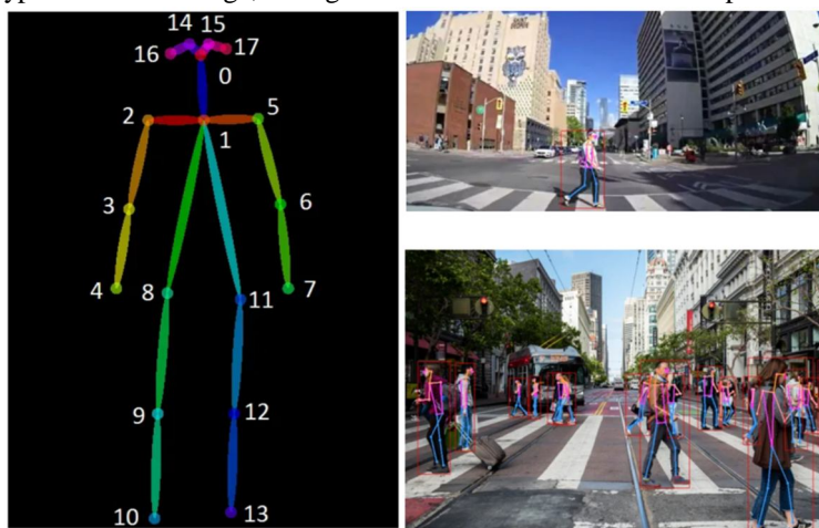
Fig. 4 Annotated Keypoints on the Test Image using YOLOv7-pose
