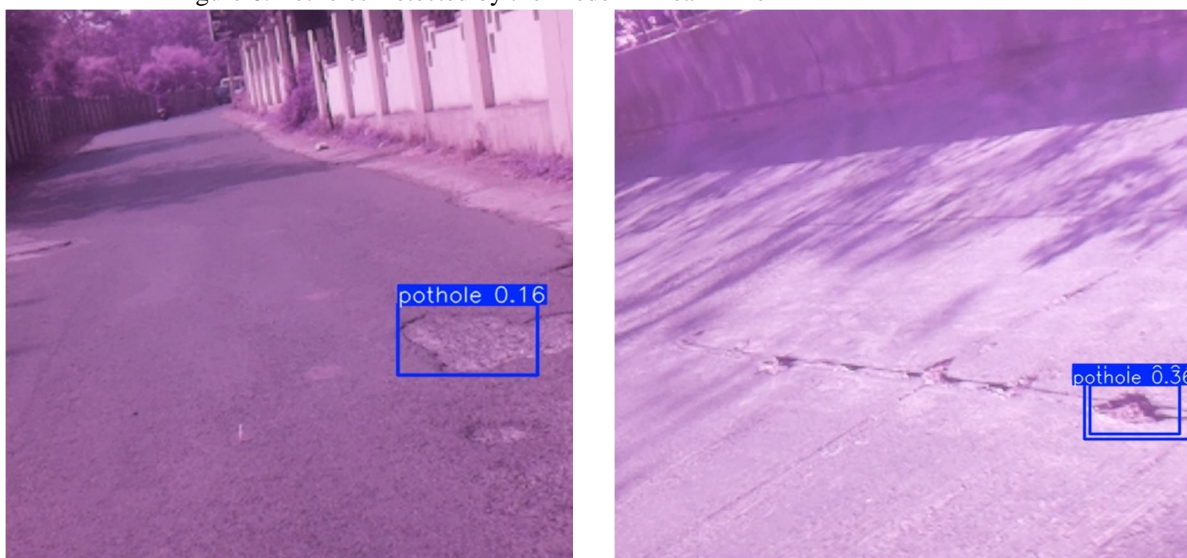
Figure 6: Potholes Detected by the Model in Real-Time
