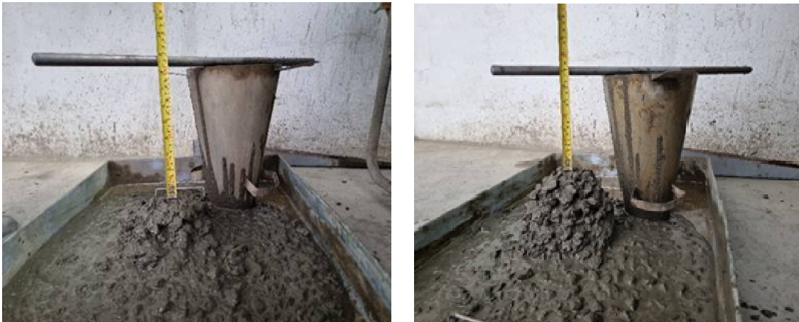
Fig-7: Slump test of concrete at 45 minute & at 90 minute.
