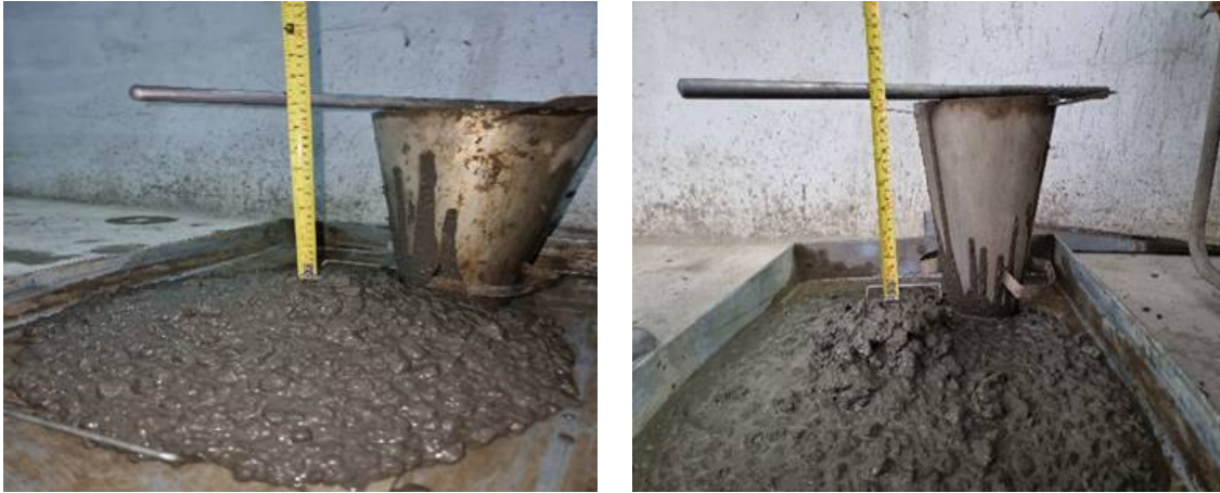
Fig-6: Slump test of concrete at immediate & after 30 minute.
