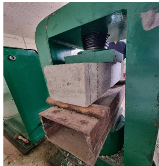
Fig-8: Compressive and Flxural test of concrete.
