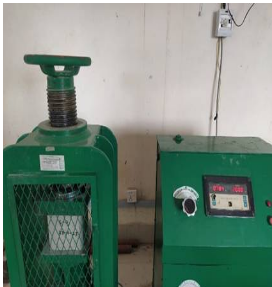
Fig-8: Compressive and Flxural test of concrete.
