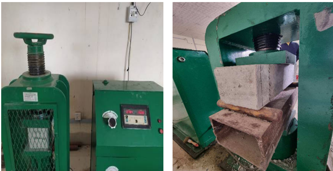
Fig-8: Compressive and Flexural test of concrete.
