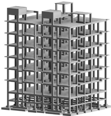
Fig 5: Structural BIM Model
