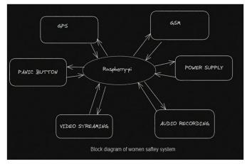
Below is a brief explanation of the modules and parts that will be used in the Raspberry Pi system: The Raspberry Pi is a controller board with an on-board 802.11n Wi-Fi network, Bluetooth, USB boot capabilities, and a 1.2 GHz, 64-bit, quad-core processor based on the Broadcom BCM2837 chip.
