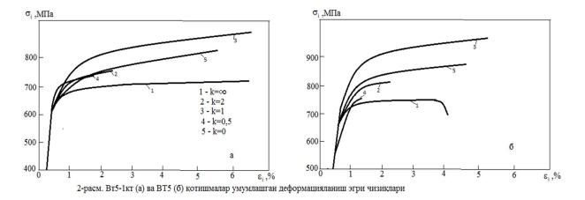
Titanium alloys Vt5 and VT5-1kt have a sufficiently high deformation ability in linear and two-axis straight elongation. This property is clearly shown in the diagrams, which show that the intensity of finite plastic deformations depends on the stress state. Both alloys have the least marginal deformations when loaded in the stress state at head ratios k = 0.5 and k = 2.
